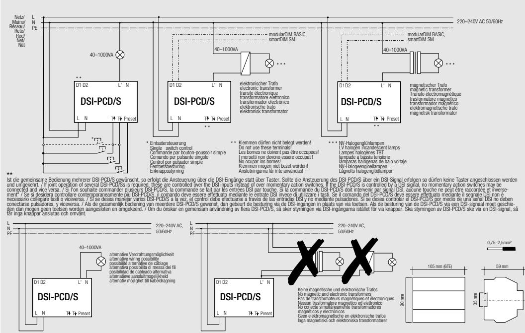
**UK** Digital phase dimmer or digital reverse phase dimmer for dimming low-voltage tungsten halogen lamps in combination with electronic transformers or magnetic transformers, and ohmic light sources with a total connected load of 40–1000 VA.
