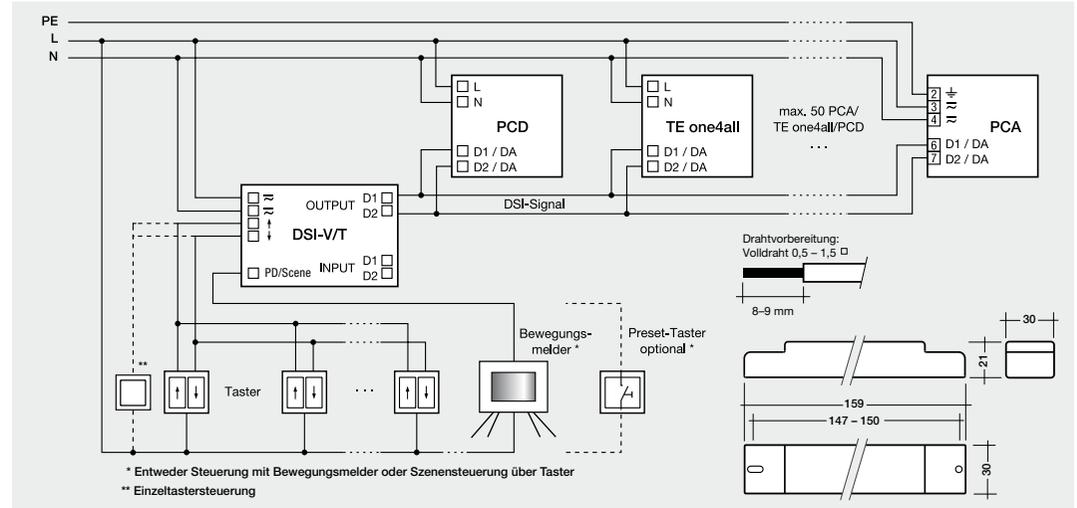
**UK** The digital DSI control module is designed to control up to 50 digital units such as electronic control gear, transformers and phase dimmers. It therefore has all the properties shared by all DSI units so far and enables PCA/TE one4all/PCD digital electronic control gear to be automatically switched and controlled via the control line.
