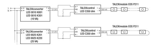
The momentary-action switch mode allows a direct connection of a push to make switch for dimming and switching. Brief push (< 0.6 s) switches ballast ON and OFF. The ballasts switch-ON at light level set at switch-OFF.
