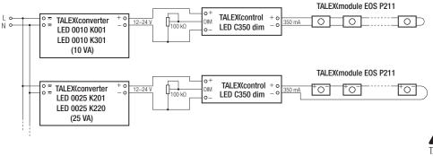
TALEXeos modules must be wired in series connection to the constant current source TALEXcontrol C350 dim
