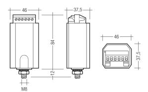
Reduces the light output of MBF and SON lamps by switching between choke-tappings, thus saving energy without reducing lamp life. Lamp manufacturers recommend that the lamp should always be started at 100 %.
