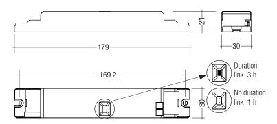
Note: LED Driver supplied with duration link in 3 hours position. Remove duration link for 1 hour duration. Duration link must be set before battery and mains connection. The EM converterLED BASIC 135 NiCd is supplied without a duration link. The duration is set to 3 hours and cannot be changed.
