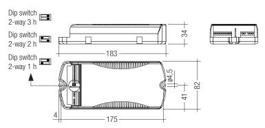
Note: LED Driver supplied with duration dip switch (2-way) in 3 hours position. Duration dip switch and I-SELECT 2 PLUG must be set before battery and mains connection.
