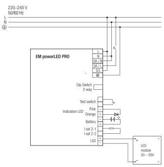
In switchDIM operation the emergency unit will work as SELFTEST unit. All functions and duration tests will perform automatically. The randomized testing is not active. For details refer to chapter 7.12 Testing, DALI Control.
