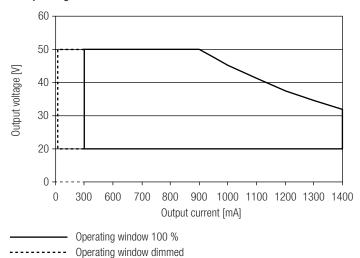
Make sure that the LED Driver is operated within the given window under all operating conditions, also in dimming operation. Otherwise certain limitations may occur. This is due to the nature of amplitude modulation dimming. The stated minimum output voltage shall not be undercut as this may cause the device to shut-down.
