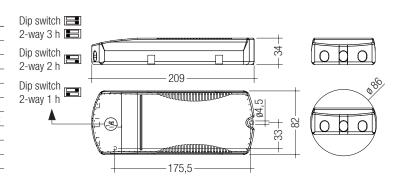
Note: LED Driver supplied with duration dip switch (2-way) in 3 hours position. Duration dip switch and I-SELECT 2 PLUG must be set before battery and mains connection.
