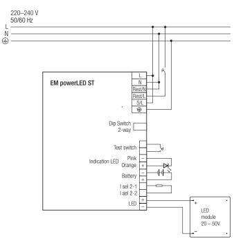
In switchDIM operation the emergency unit will work as SELFTEST unit. All functions and duration tests will perform automatically. The randomized testing is not active. For details refer to chapter 7.9 Testing, DALI Control.
