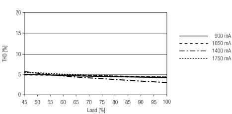
100 % load correspond to the max. output power (full load) according to the table on page 2.
