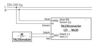
Secondary switching of LEDs is not allowed and may cause damage to the LEDs. The hot plug-in of LEDs during normal operation may result in current peaks of up to 50% above the typical output current.
