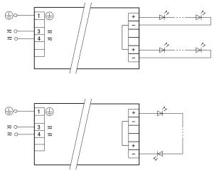
LED's have to be connected as shown above to work properly. It is possible to connect a different number of LED's on two circuits (like on top picture). The minimum power load has to be connected. Otherwise the LED Driver will switch off.
