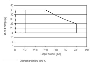
Make sure that the LED Driver is operated within the given window under all operating conditions. Special attention needs to be paid at dimming and DC emergency operation as the forward voltage of the connected LED modules varies with the dimming level, due to the implemented amplitude dimming technology. Coming below the specified minimum output voltage of the LED Driver may cause the device to shut-down. See chapter "6.11 Light level in DC operation" for more information.
