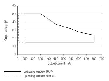
Make sure that the LED Driver is operated within the given window under all operating conditions. Special attention needs to be paid at dimming and DC emergency operation as the forward voltage of the connected LED modules varies with the dimming level, due to the implemented amplitude dimming technology. Coming below the specified minimum output voltage of the LED Driver may cause the device to shut-down. See chapter "6.11 Light level in DC operation" for more information. 4.4 THD vs load
