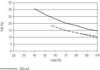
$100\ \%$  load corresponds to the max. output power (full load) according to the table on page 2.
