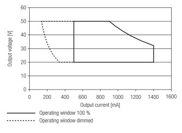
Make sure that the LED Driver is operated within the given window under all operating conditions. Special attention needs to be paid at dimming and DC emergency operation as the forward voltage of the connected LED modules varies with the dimming level, due to the implemented amplitude dimming technology. Coming below the specified minimum output voltage of the LED Driver may cause the device to shut-down.
