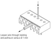
and pulling or using a Ø 1 mm release tool
