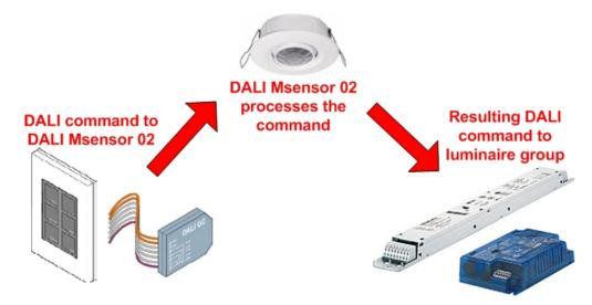
Like DALI control gear, the DALI MSensor 02 reacts to commands that are sent to it, i.e. commands sent to its DALI address, DALI group (luminaire group), or to broadcast commands.
