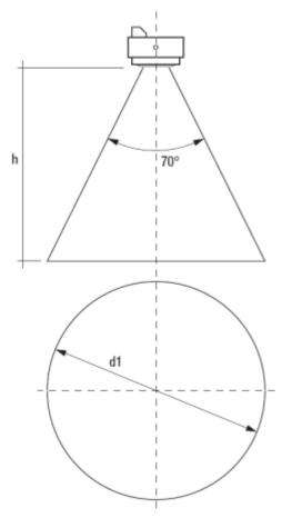
The diameter of the detection area depends on the detection angle of the sensor and the height at which it is mounted.
