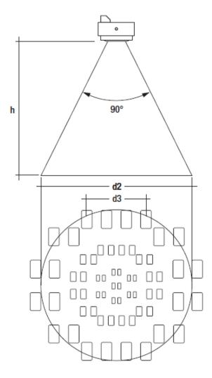
The diameter of the detection area depends on the detection angle of the sensor and the height at which it is mounted. The mounting height also has an effect on the sensor's accuracy.
