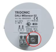
The effective range of the DALI MSensor 02 is set using the rotary switch at the rear of the sensor. All control gear located within the previously set effective range is controlled by the sensor.
