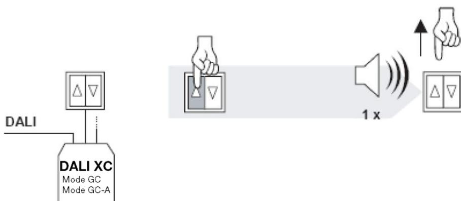
Figure 9: Assigning a luminaire to a group
