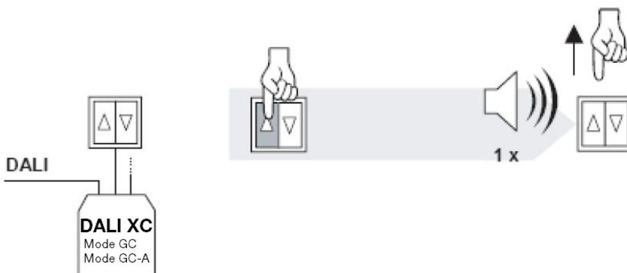
Figure 5: Assigning a luminaire to a group
