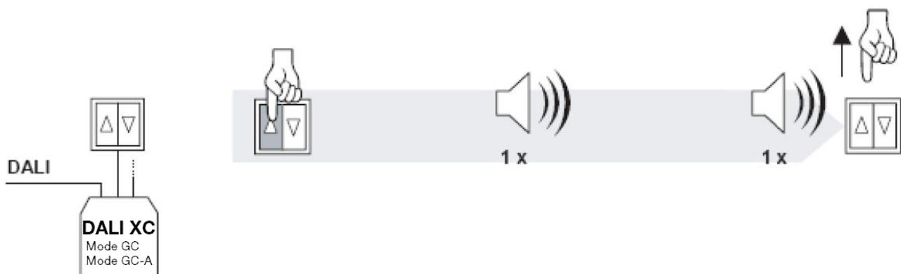
Figure 8: Deleting a luminaire from a group
